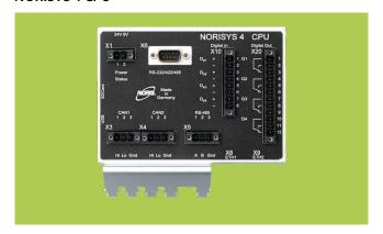
Programmable logic controller according to the IEC 61131 standard featuring a 32-bit, 400 MHz processor and integrated web server. An optional data logger function can store up to 32 GB of data on SDHC cards.
