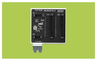
Process interface unit with 24 digital channels which can be configured as inputs or outputs via software. All channels are short-circuit proof and can drive up to 0.5 A.
