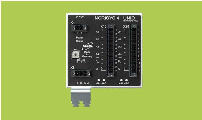
Process interface unit for universal input-output processing which can be expanded by using different signal cards. Two module slots can be equipped with cards for analogue standard signals and temperature measurement as well as for custom cards. Each analogue standard signal channel can be configured as a 0...5 V, -5V...+5 V, 0...10 V, -10 V...+10 V, 0...20 mA or 4...20 mA channel.
